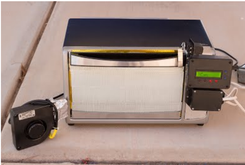
Blower on the Left, Relay Module is in added enclosure below ControLeo2
