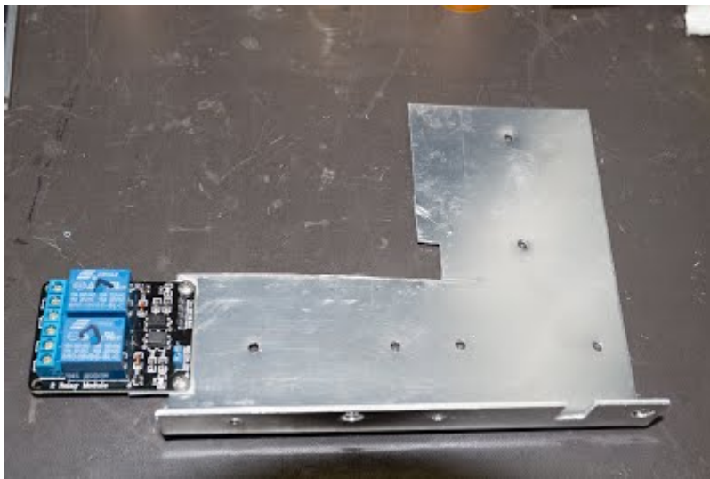
Dual Relay Module mounted on Solid State Relay Support
