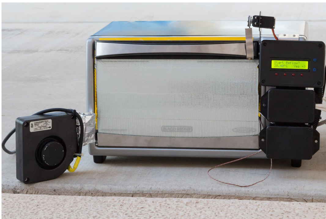
Completed Reflow Oven
