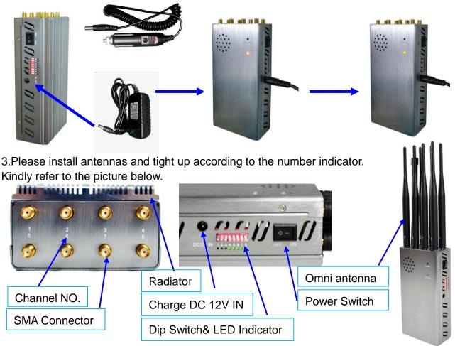
4. Turn on the power switch and the Power LED shall light in Green and the LED of each band will turn on too.
