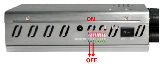
The number indicators are corresponding to the number of antennas, LED turns on which indicate operating.
